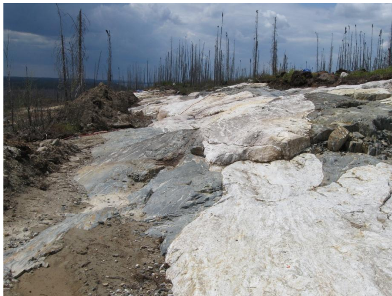
Figure 12: Stripped trench at Whabouchi, showing the pegmatite (white) cutting its oligoclase gneiss host (dark grey). Field of view is approximately 15 m. Photo from Nemaska Exploration Ltd.
