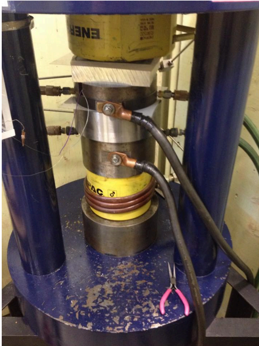
Figure 5: An experiment running in the piston cylinder. The two black cables are power leads and the silver disk in between is the pressure vessel, where the sample is located.
