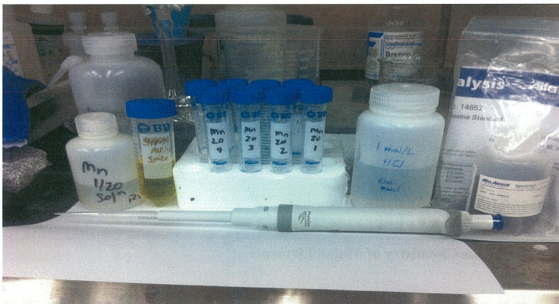
Figure 5: From left to right, Mn(1/20) solution (melt from Mn 1/20 experiment dissolved in 100 mL 1 mol/L HCl); 5 ppm Au/Ir spike; 4 falcon tubes (containing 5 mL of Mn(1/20) solution, and 0 – 50 ul of 5 ppm spike); 1 mol/L HCl; Alfa Aesar 100 ppm precious metals standard solution.
